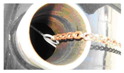
Clean the interior of the fuel neck with the POR-15 Metal Ready product. Spray a clean rag with the cleaner and swab the interior of the neck to remove any loose rust. Be careful not get any of the cleaner or rust into the tank.
