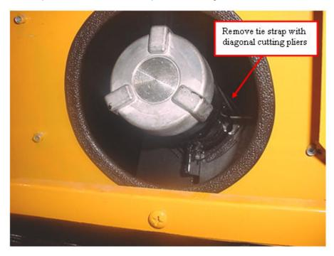
Cut the tie strap loose and remove from the fuel neck.
