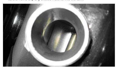
When correctly applied, the fuel neck should have an even silver appearance.
