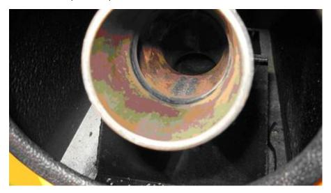
If rust is present, locate the tie strap that is holding the neck into the receiver.
